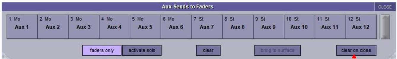
When the panel is closed, sends to faders is canceled reverting the faders to channel level.
